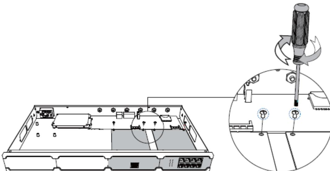
**STEP 5** Insert the Telephony Modules on the EX08 Board. Skip this step for EX30 Board.
