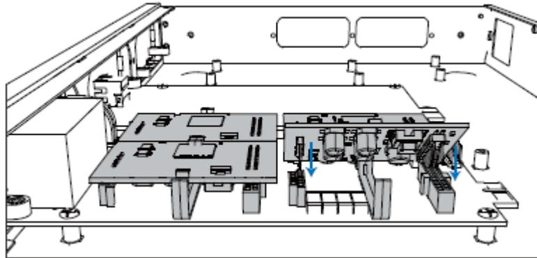
**STEP 6** Insert a SIM card on the GSM/3G module following the instructions. Skip this step if no GSM/3G module installed.
