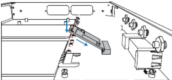
**STEP 2** Lock the screws to fix the D30 module board.
