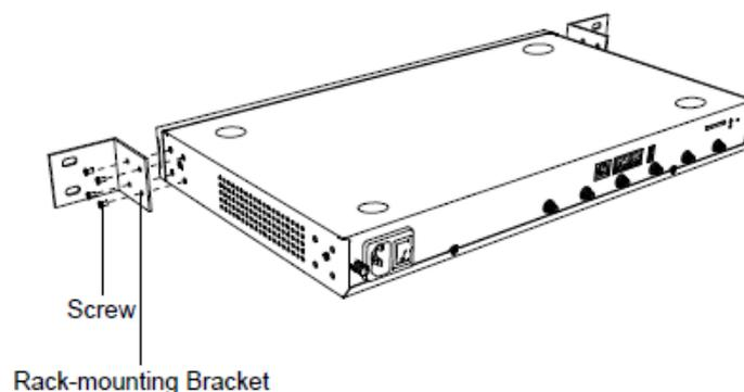
**STEP 2** Place the PBX in the 19-inch rack and fix both brackets to the rack with the rack's proprietary mounting equipment.
