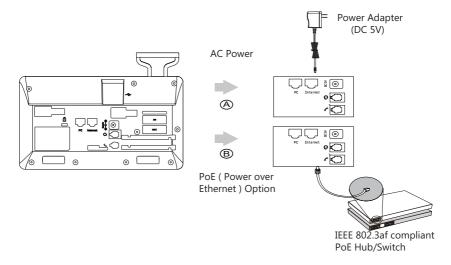
**Note**: The IP phone should be used with Yealink original power adapter (5V/1.2A) only. The use the of third-party power adapter may damage the phone.
