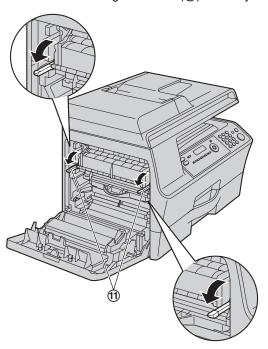
2. Remove the jammed paper (②) carefully by pulling it rightward.
