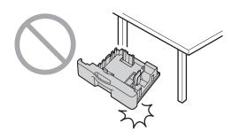
Hold the standard input tray with both hands when removing or installing. The standard input tray weighs approximately 4.8 kg (10.6 lb) when fully loaded with recording paper.
