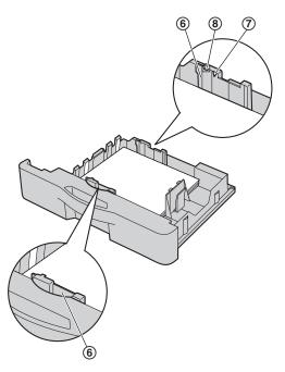
Insert the standard input tray into the unit, lifting the front part of the tray. Then push it completely into the unit.
