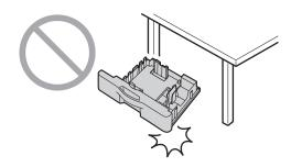
Hold the optional input tray with both hands when removing or installing. The optional input tray weighs approximately 4.8 kg (10.6 lb) when fully loaded with recording paper.
